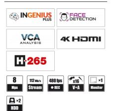
•16 x video and audio channels •Recording speed up to 480 fps at 3840 x 2160 •Supports resolution up to 3840 x 2160 •Recorded stream size: 112 Mb/s in total from all cameras
