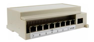
The **NVE-SW200-7P** switch is a device intended for communication of other NVE system devices, i.e. input panels with monitors. Seven ports allow you to connect and power with sPoE 18VDC a group of devices and an additional UP-LINK port allows you to connect another switch if needed.
