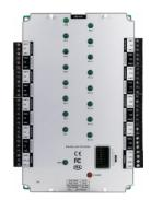
Extension module KDH-MOD2016-ELV increases the number of floors supported by the controller KDH-KS2000-IP-ELV. Using 4 modules of this type enables to control up to 69 floors by one elevator controller.
