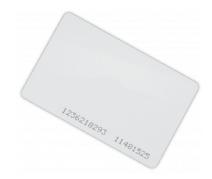
Proximity card, dual. It operates on frequencies of 13.56 MHz and 860 MHz. Designed for cooperation with Mifare card readers (eg KDH-C100M) and long-range readers working in the UHF band (eg KDH-CDZ900). It is worth noting that the number printed on the card is the same for both versions (Mifare and UHF), which makes it easy to add it to the system using the USB administrator card reader - KDH-CADM-M32. The card is of the PVC type and has the option of printing the photo-ID.
