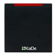
Proximity card readers type KDH-C110U can be installed inside or outdoors. They have housing made of ABS plastic. Readers are designed to work with controllers with Wiegand interface. The devices reads the card Unique (125 kHz). Switchable Wiegand format makes this product universal for various installations. The range of the proximi-ty card reading is from 2 to 10 cm depend of the model and type of card.
